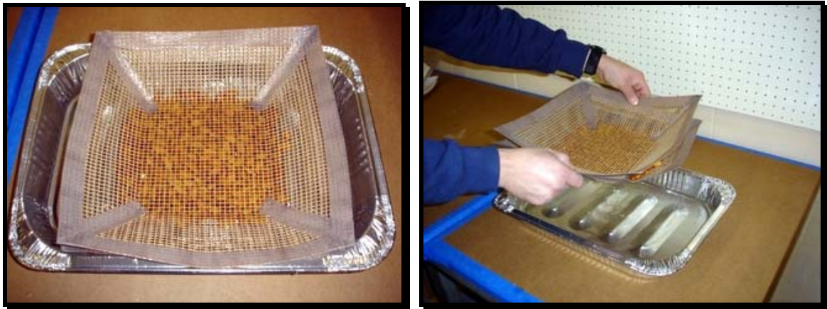
Figure 10a & b: Almonds submerged in water between two mesh carriers and then shaken to remove excess surface water
