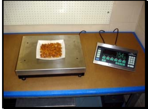
Figure 7a & b: Verifying target weight and filling bottom layer of test carrier with half of the uninoculated almonds
