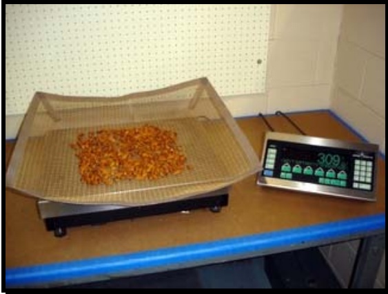
Figure 7a & b: Verifying target weight and filling bottom layer of test carrier with half of the uninoculated almonds
